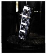
A hot jet spray wash is commonly used to clean blocks, cylinder heads, crankshafts, and more. The table rotates as high-pressure heated solvent or detergent is sprayed.
