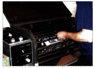
An airless shot blaster slings steel (or stainless steel) shot onto the block or cylinder heads as the part is rotated while secured in an adjustable cage. Compressed air is not used. Following shot blasting, the part must be tumbled in a rubber-lined drum to shake any remaining steel shot from the part.
